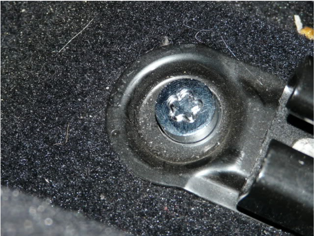
Gorilla Installed. Seats all the way in just fine and the head of the bolt is only slightly smaller than the oem washer.
