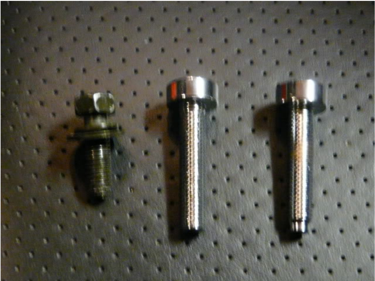
From left to right you have the stock bolt, Gorrilla Bolt, and McGard Bolt. As you can see the main difference is the the bottom of the bolts which really didn;t make a difference when installing them
