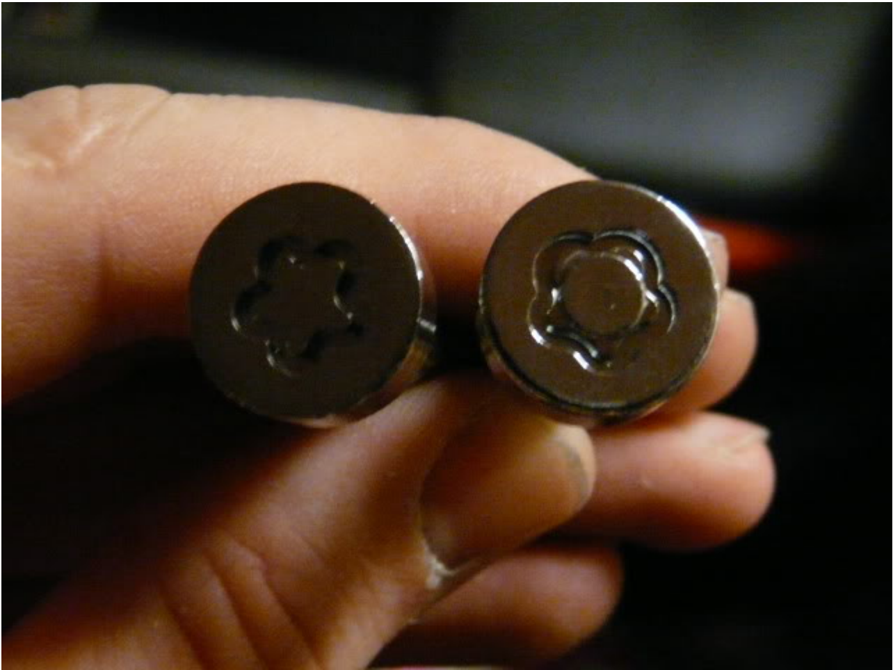
Gorilla is the Left McGard on the right As you can see they are slightly different and something to note is that the tools are not interchangeable.
